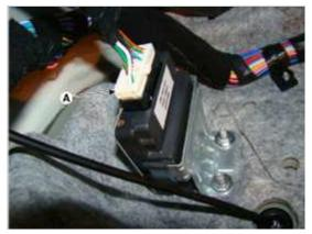
4. Loosen the nuts (A) and then remove the 4WD ECU.
