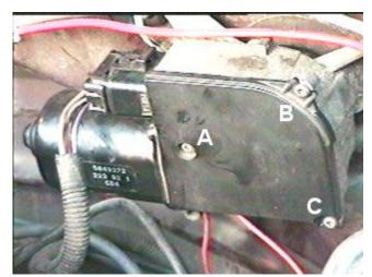
I decided to look at mine...the hard way. I removed the entire wiper unit, which involves taking some plastic off up near the windshield, and disconnecting the wiper mechanical and electrical linkages, plus some bolts, screws, etc. The EASY way, as I learned later, is to just remove the three screws holding the circuit board cover. Actually, you only have to remove screw A, and just loosen B and C, since the corners are slotted, rather than holes. The are Torx head.
